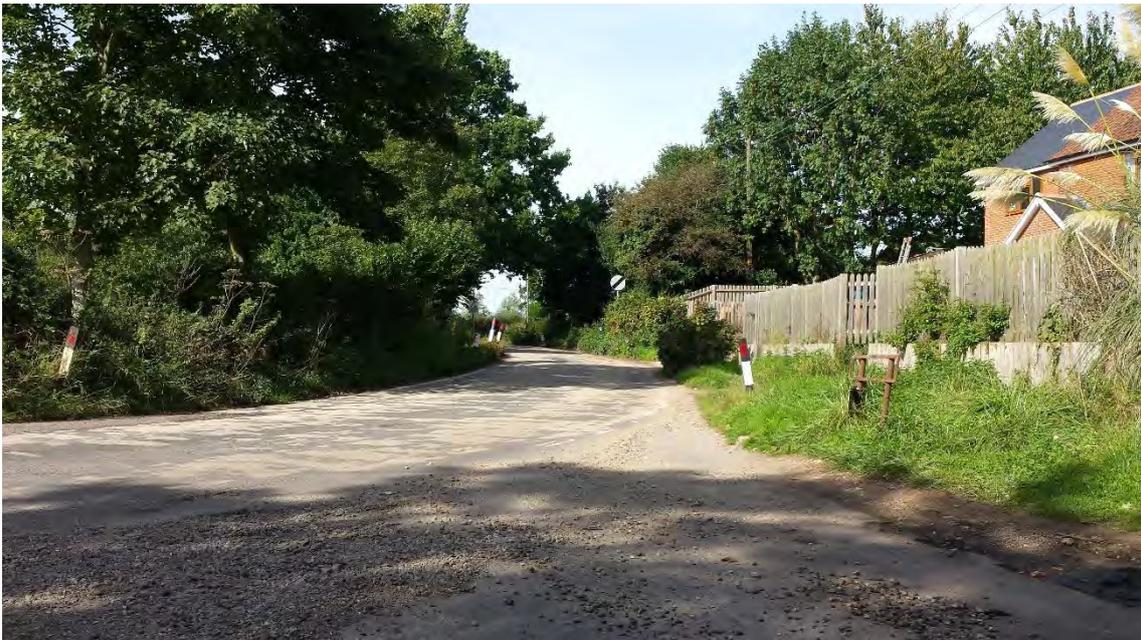
This surfacing has been installed to provide an increased skid resistance on the bends and as there are not any personal injury collisions recorded at either bend it appears to be working.
