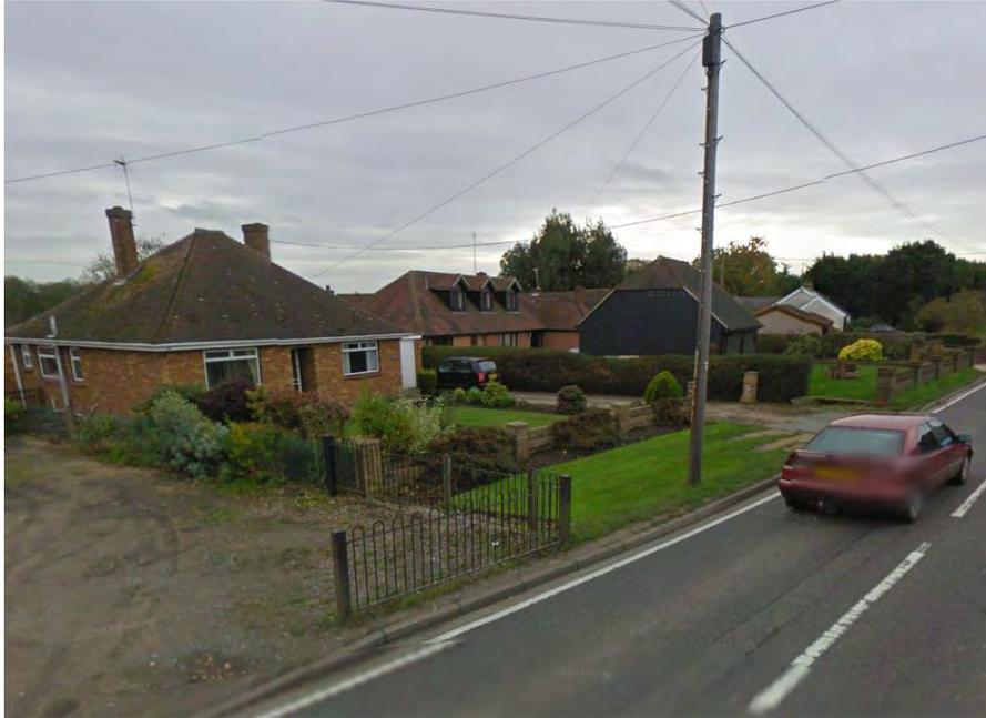
This property has a boundary wall set back approximately 5m from the carriageway, however there is a BT pole set back 0.75m back from the kerb face. A shoot gully with associated access chamber is also present.
